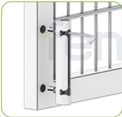
Align the holder with the holes in the gate leaf and insert the expanding nuts. Tighten the nuts with an Allen key.
