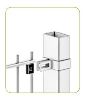
Make sure the lower bracket is above the twin bar and attached to the fence. When placing the bolts, take into account the direction in which you insert the bolt. Make sure that the nut cannot be loosened from outside the fence.
