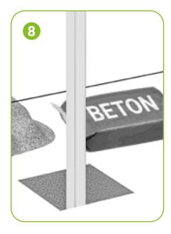
Dig or drill a hole of approximately 30 x 30 cm where the first post is to be placed. Remove any stones, roots or other material from the ground where the posts will be placed.
