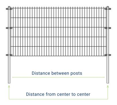
\*Center to center is the distance between the center of one object and the center of the other object. So from the center (middle) of the first post to the other center (middle) of the second post.
