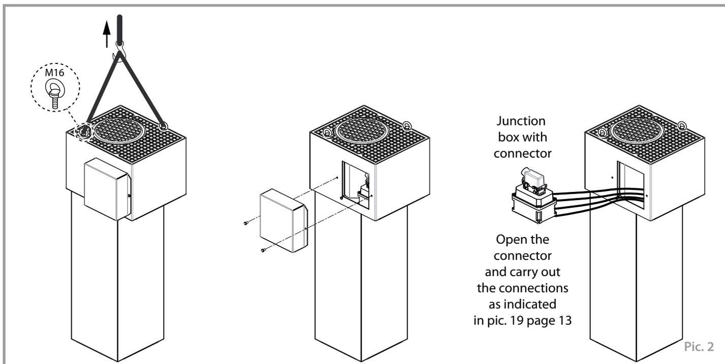
REMOVING THE BOLLARD FROM THE CASING
