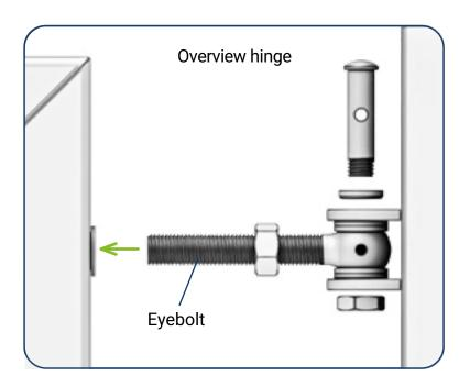
Pre-adjust the hinges to ease assembly later. Tighten the nut on the eyebolt and then tighten the eyebolt into the gate wing. Do not tighten the nut against the gate leaf yet. Turn the eyebolt in the same number of turns on both hinges.
