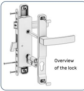
Slide the lock case into the leaf and tighten with the Allen key. Now push the latch with the cover plate together with the cylinder lock in the case and screw the cover plate with the screwdriver. Turn around the latchbolt:
