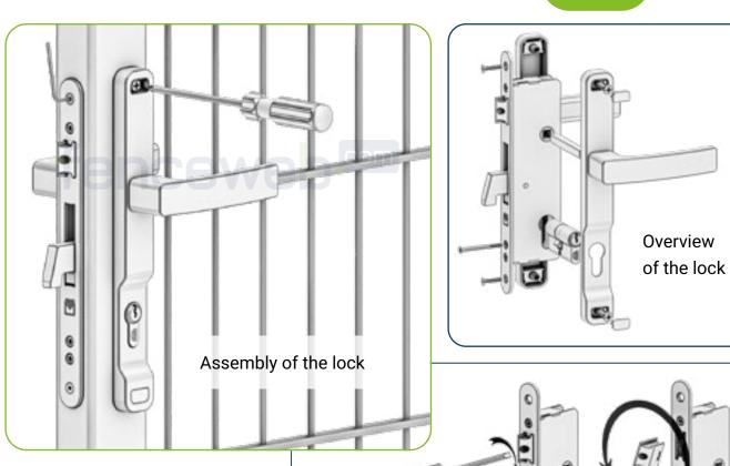
Slide the lock case into thewing and tighten with the Allen key. Now push the latch with the cover plate together with the cylinder lock in the case and screw the cover plate with the screwdriver.
