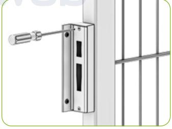
Make sure that you mount the striker correctly in relation to the direction of rotation of the gate.
