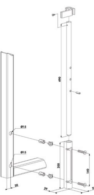
Lay down the parts of the drop bolt and check if all parts are present.
