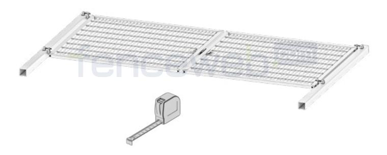
Lay out the gate parts on a soft surface and measure them.
