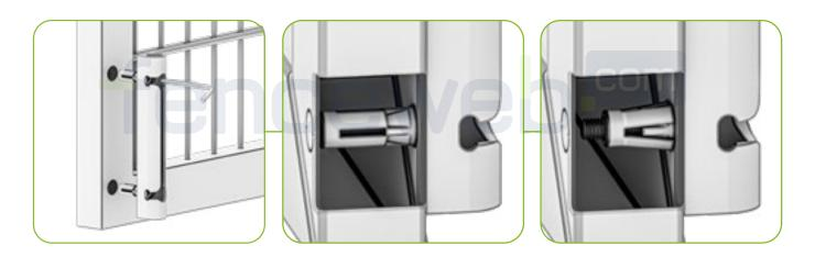
Allign the holder with the holes in the gate leaf and insert the expanding nuts. Tighten the nuts with an Allen key.
