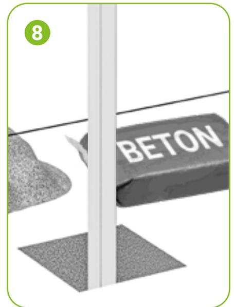
Secure the post with (quickdrying) concrete. For fencing higher than 1 meter, we recommend to always secure the posts with (quickdrying) concrete. Follow the instructions on the packaging. Let the concrete harden before mounting the fencepanels.
