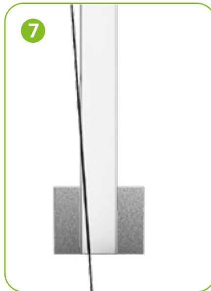
**Place the post in the hole.** Check if it is level and place it against the stretched wire. Then bring it into the ground to the correct height. Use one if necessary a post driver. The round post generally goes 80 cm into the ground. We recommend keeping the fencing minimal 5 cm above ground level to place.
