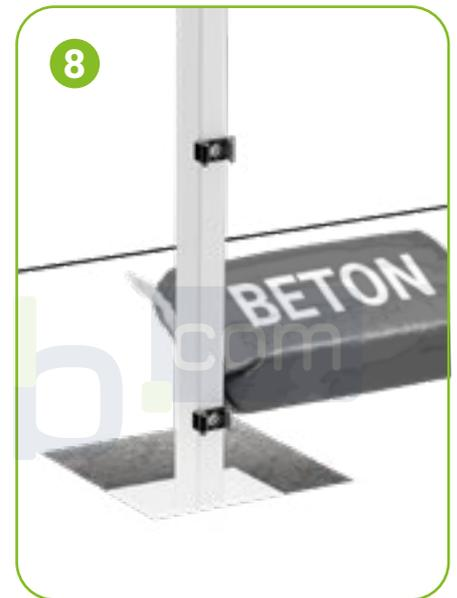
If necessary, secure the post with (rapid) concrete. For fences higher than 1 meter, we recommend always securing the posts with (quick) concrete. Follow the instructions for use on the packaging. Repeat after installing the first post the procedure for all posts. Let the concrete harden before applying mounting the fencpanels.
